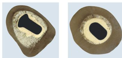
Manto de cemento BiCONTACT® proximal y distal
