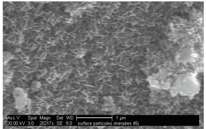
Scanning Electron Microscope characterisation of the mineral layer formed on GlassBONE™ granules.
